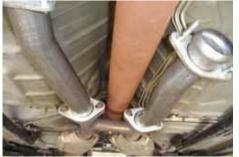
Start by removing your stock exhaust system. Once removed install both flow tubes as shown. Do not tighten.
