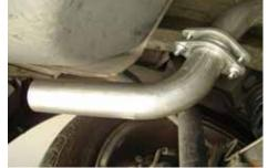
Install both of the down tube to the MAC mufflers as shown. Do not tighten. Note: Both of the down tubes are the same.
