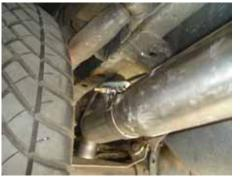
Align both tips and tighten. Start and check for leaks.
