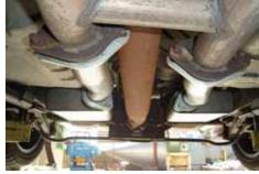
Align the MAC exhaust system and tighten starting at the flow tubes.
