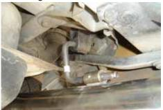
Install the hanger into the stock location and slide the tip into the down tube then the hanger as shown.
