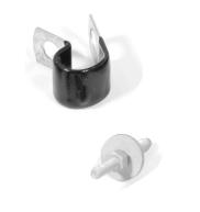
Flanged/Studded Bolt - This bolt is installed on the EVAP solenoid, and has the extended, threaded stud, to allow the factory wiring harness retainer to be reinstalled. While standing at the front of the vehicle, this bolt will be installed on the right side of the EVAP solenoid. Encluded is the wiring/hose retainer. This can be used on the studded bolt to retain the vacuum hoses and prevent the hoses from moving.
