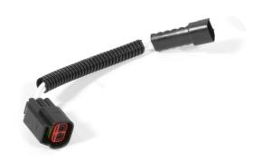
EVAP Extension Harness - The extension harness included is designed to extend the wiring harness to accommodate the different orientation of the EVAP solenoid. This extension plugs into the factory wiring harness, and does not require cutting.
