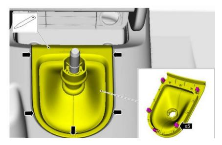
**STEP 4:** Release the retainers and remove the gearshift lever boot.
