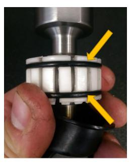
**STEP 19:** Apply a liberal amount of the supplied grease to the shifter shaft pivot and into all the voids on the shifter pivot bushing. Articulate the bushing around to ensure grease has completely covered the shifter shaft pivot.
