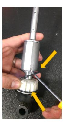
**STEP 12:** Utilizing the steel pin removed in Step 8 or a suitable punch, gently tap the shifter pivot bushing to remove from the shifter handle assembly.
