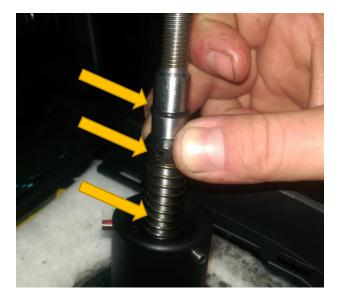
**STEP 29:** Using a suitable punch, tap the provided roll pin through the anti-rattle washer until it is centered within the shifter handle.
