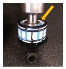
**STEP 21:** Slide the new shift handle assembly into the shifter housing. Verify that the upper shifter bushing rubber isolator stays in position as the assembly is installed.
