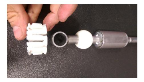
**STEP 15:** Install the shift handle pivot bushing onto the new shifter shaft by sliding it over the lower portion of the shifter shaft and gently pushing upwards until it is positioned over the pivot ball.
