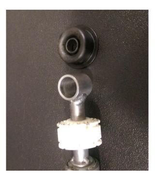
**STEP 14:** Remove the shift handle pivot bushing by gently pushing downwards until it is released from the pivot ball. Slide the bushing over the lower pivot to remove completely.
