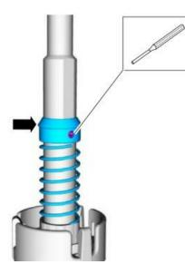
**STEP 6:** Remove the reverse lockout collar.
