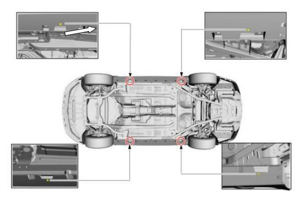
WARNING: Identify the correct jacking points by locating the triangle stamped into the unibody sheet metal or vehicle frame. Raising a vehicle in any other location may result in vehicle shifting or falling. Failure to follow this instruction may result in serious personal injury.
