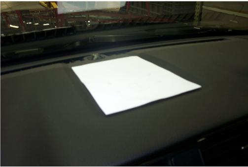
Note: A standard drill does not fit in the space between the dash and the windshield. It is recommended that the installer use a small 90 degree drill or a tool like a Dremel to make the required holes. Alternatively, a 1/4" 90 degree die grinder with a 1/8" collet adapter works well
