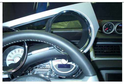
**Step 3:** Prepare Instrument Panel (IP) for installation of gauge pod mounting bracket. Use the template on last page of these instructions to locate the 4 holes necessary for connecting the gauge pod mounting bracket to the IP.
