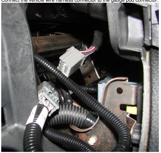
**Step 8:** The takeout for the oil pressure sender routes through the large grommet in the driver's side foot well. Identify the service nub in this large grommet just inboard of the OEM wiring harness. Remove a small portion of this nub as required to permit pass through of the wire harness.
