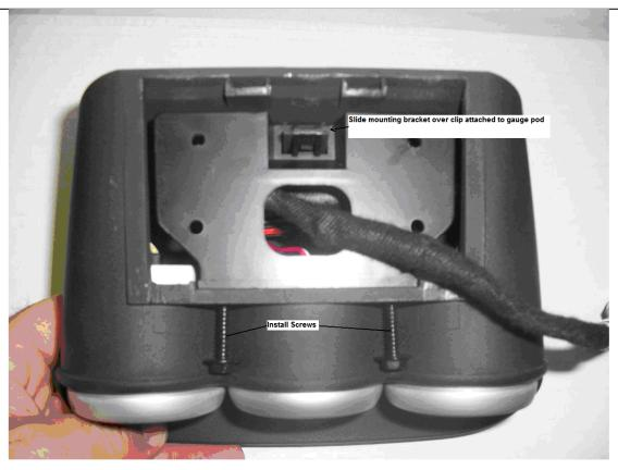
**Step 6b:** Install remaining two screws through front of gauge pod to secure installation of the pod to the mounting bracket.
