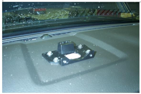
**Step 6a:** Pass gauge pod wire harness through IP dash pad and mount the gauge pod to the mounting bracket by sliding the clip on the back of the gauge pod into the socket of the mounting bracket (refer to picture below).
