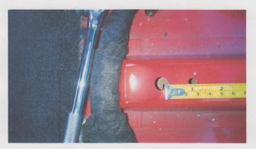
There are 10 stripes of Velcro in your kit. Place a strip on the top & bottom left and right as shown. Also, place a Velcro in the center of the top and across the front bottom at the floor carpet.
