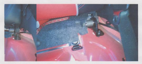
Once the nuts are removed, the rear backrests can come out by pulling the cloth tab to release the backrest catch and then lifting the outboard end off the stud and pulling the center off the mount as shown below.
