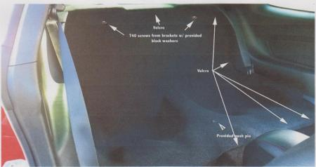
The rear seat delete is retained by two bolts & one push pin. Two of the three will go into factory threaded holes on the vertical area of the package shelf where the seat back retainers were removed as shown. The third is the new hole drilled in the floor area. The provided large trim clip, often referred to as a "Christmas Tree clip" should be used to retain this portion of the delete kit.
