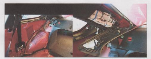
Rotate the trim to remove it from the pillar and expose the pillar components as shown.
