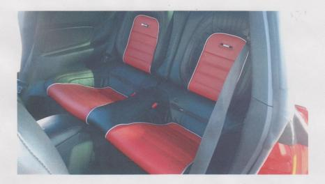
First, you will need to remove the rear seat lower cushion and two backrest cushions. To remove the lower cushion, push the front of the seat bottom toward the rear and lift. This will remove the clip from the hole in the floor. Do this on the left and right sides. When up as shown above, lift the bottom cushion out and remove from the car.
