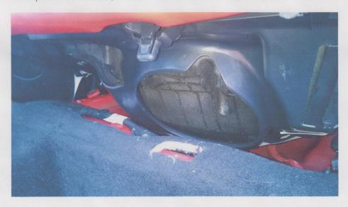
Once the bottom is out, remove the left and right backrest cushions by removing the nuts on the left and right of car where the bracket is bolted to the floor. This requires a the 15MM deep well socket.
