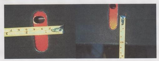
On the floor, drill and  $\frac{1}{4}$ " hole 1" toward the rear of the car from the large hole just aft of the floor carpet.
