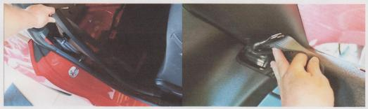
Before you remove the quarter panel trim pieces, unclip the seat belt trim plastic and slid it out of the way. This will give you access to the belt assembly. Un snap and remove the quarter trim as well as the C pillar trim.
