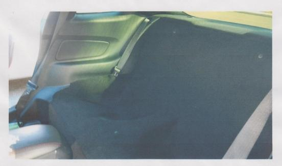
The biggest downside to this install is caused by the removal of the rear seat belts. If you want to reuse the OEM seatbelt trim to keep the interior looking tidy where the rear seatbelt pass through the rear trim panels, you'll have to cut the belts. Ford does not offer this as a separate service part, and the only way it will separate it from the seat belt is to cut it or the seat belt.
