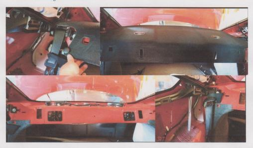
Removal of the seat belt assembly involves the removal of 3 bolts. Two are exposed and the third is behind the black trim below the window. Pull it away from the body a little and you can get the socket on the third bolt. Use your T40 to remove the two rear backrest retainer brackets. You will reuse the outboard bolt to hold in your new RSD.
