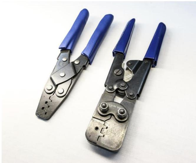
4. With the terminal in the crimper, insert the wire/seal into the terminal. The end of the bare wire should end up even with the part on the terminal that will crimp it. When aligned, crimp
