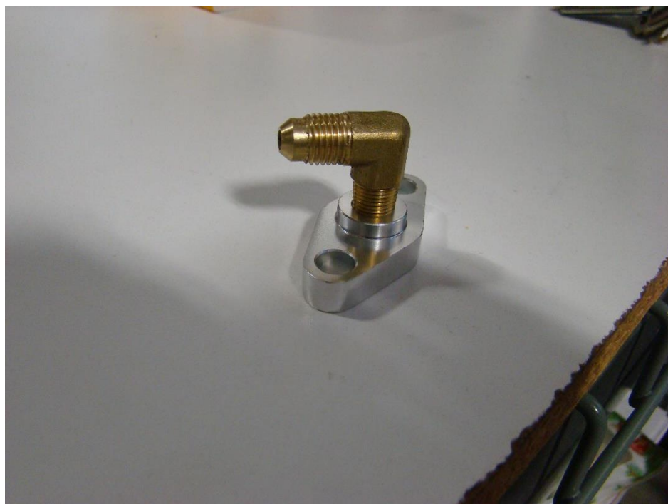
Oil Feed at the turbo
