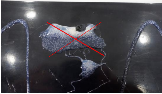
Figure 2. Avoid glue pooling.
