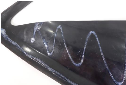
Figure 1. Thin glue pattern.
