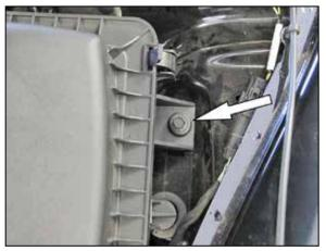
8. Remove the bolt securing the air filter assembly onto the inner fender.
