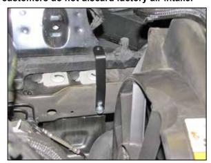
10. Install the heat shield mounting bracket (064325) onto the inner fender as shown using the provided hardware.
