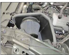
15. Install the K&N<sup>®</sup> air filter onto the adapter and secure with the provided hose clamp then secure the heat shield to the air filter housing mounting location using the provided hardware.
