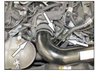
21. Connect the crank case vent, EVAP vent and idle by pass lines to the quick disconnect fittings installed into the K&N® intake tube.
