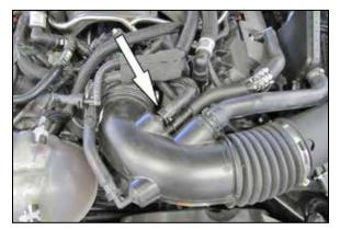
3. Depress the locking tab and then disconnect the idle bypass hose from the intake tube.
