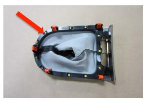
Turn your boot over and locate the small circular welds found on the perimeter of the underside (marked by the red arrow in the illustration). We will be removing these in the next step with a drill. Be sure to either tape over the surface of your trim ring or lay the assembly on a soft surface to prevent any scratching on its finish.
