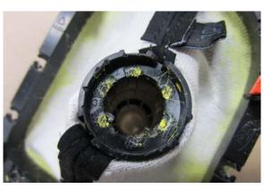
With the boot turned inside out, insert the metallic upper collar back into the black collar being careful to line up all of the pegs. The small molding lines in the metallic collar will line up with the seams on the boot. You may need to put the metallic collar down on a flat surface and either gently tap the black collar down to lock it in or push it with your hands. The fit should be tight enough to form a secure hold but you may use adhesive to hold the two together if needed.
