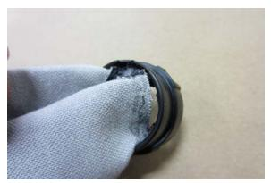
Remove the top of the boot from the black trim ring. It should peel apart by pressing the boot inward from the plastic ring.
