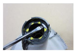
In this picture, you can see each section broken free. At this point you can wiggle the black collar apart from the upper collar.
