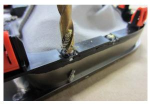
Using the slow speed setting on your drill or being careful not to spin it up too fast, start drilling the plastic rivets on the bottom of the trim ring. You only need to shave off the top of the rivets. Be carful not to drill down into the trim piece itself. Sharp/new drill bits will want to pull down into the trim ring. This step can also be accomplished with a small Dremel grinder to grind the rivets down.
