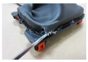
Remove the top metal finished trim ring and peel the vinyl boot from the black plastic ring. The flat head screwdriver helps here as well. Remove any remnants of the old boot behind as they may cause the new boot to not fit properly.
