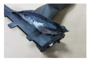
Peel away the boot from the trim ring. You may need a small flat head screwdriver to help get the edges started.
