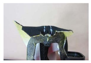
Adhere the back seam to the trim ring. The back edge of the boot should stop halfway down the wall of the trim ring.
