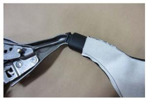
Turn the boot inside out and slide it over the parking brake handle.
