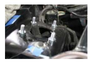
14. Assemble the bearing cup onto the caster/camber plate as shown with the supplied J&M bolts and washers. Leave bolts loose for now to allow for easy adjustments.
