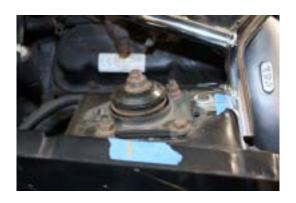
2. Place the front end of the car on jack-stands and remove wheel. This will allow access to the strut mounting bolts. Place a floor jack under the front lower control arm such that it applies a small amount of lift on the lower control arm.
