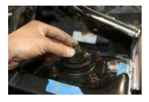
3. Many 94-04 Mustangs are equipped with ABS brakes. If your car has ABS brakes, begin by loosening and removing the ABS bracket mounting nut that attaches to the strut. If your car does not have ABS, you can skip this step.
