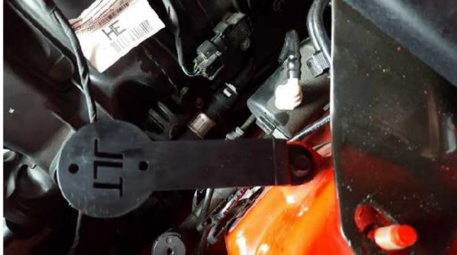
Use the supplied screws to mount the JLT Separator assembly to the JLT bracket routing the front hose under the intake for the fitting behind the throttle body and the rear hose down toward the engine mount.
