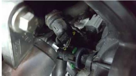
From under side route rear hose to PCV connection on the engine block
