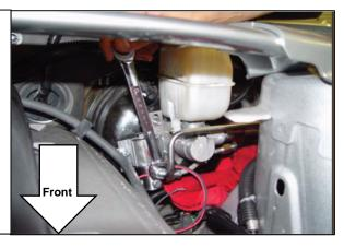
12. Thread nut back onto master Cylinder stud, tighten Master Cylinder nut to 25Nm (18ft.-lbs).
