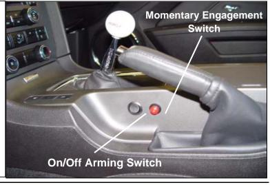
22. Reconnect battery and turn ignition switch to the "ON" position. While still in park and NOT depressing your brake pedal, activate and engage your Hurst Roll/Control system (make sure you can hear the clicking of the solenoid) several times and check fuse. If fuse is burned, check all electrical connections for a short and correct any problems immediately.
