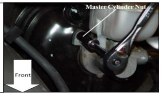
6. Remove nut/clip in order to remove OEM Induction Tube.
