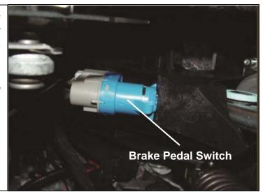
18. The brake pedal switch has a 4 wire connector — violet/red, black/blue, yellow/green, and violet / white. Remove some electrical tape and convoluted sleeve in order to have enough exposed violet/white wire to use provided Scotchlok connector (be extremely careful not to cut wires).
