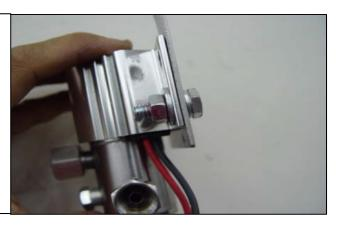
3. Tighten the provided adapters and plugs to solenoid as shown.
