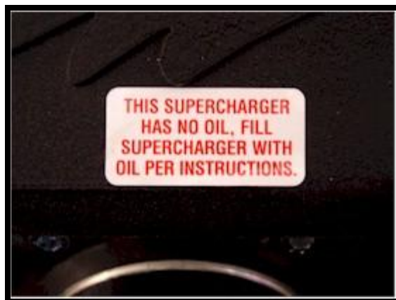
Warning label attached to Supercharger housing
