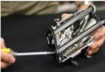
2. Next, remove the two screws holding the LED panel to the reflector housing and remove the factory LED panel. The factory panel and driver board will no longer be used.
