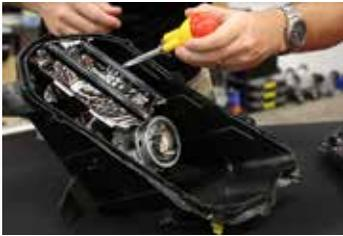
1. Remove the factory LED panels by unscrewing the screws holding the reflector housing in place and then unclip the wire connector.
