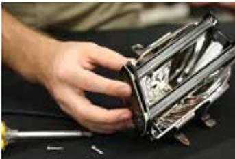
3. Place the new Diode Dynamics LED Module into position. Use the original screws to secure in place. **DO NOT OVERTIGHTEN.**
