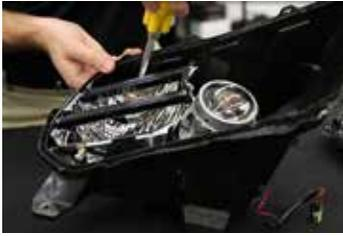
4. Using the alignment tabs, reinstall the reflector housing into main headlamp housing, running the wiring through the dust cap and resealing any holes that you may create. Replace the lense and repeat for other headlamp.
