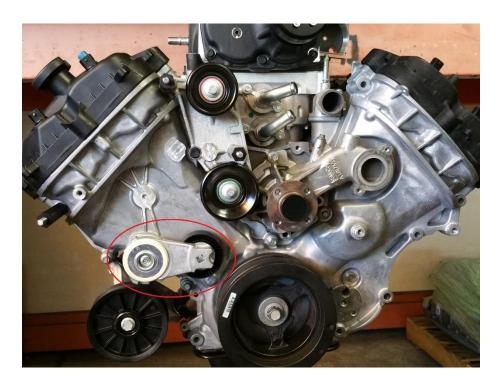
10. Assemble the alternator bracket by attaching the alternator, 1.85' spacer, 2.5" idler stand-off, hardware, and 3" idler (supplied with supercharger kit) as illustrated below. When inserting the 1.85" spacer it may be necessary to press the alternator slide nut out slightly to gain clearance.
