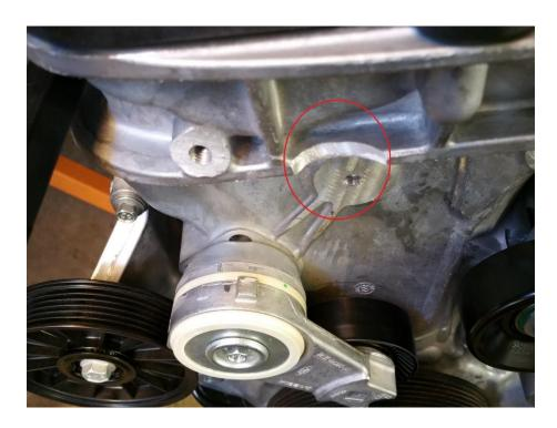
4. Remove the two timing cover bolts as illustrated below.
