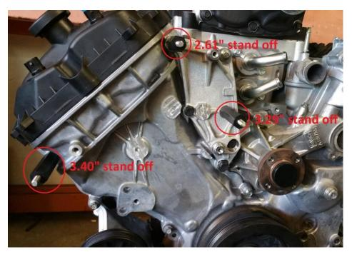
8. Install the 3.5" idler pulley (supplied) on the lower boss of the FEAD bracket. The 3" pulley supplied with the supercharger kit that would normally be installed here will be used in step # 10.
