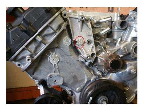
6. Install the FEAD bracket as per your supercharger instruction while leaving out the two bolts marked with an X in the illustrated below.
