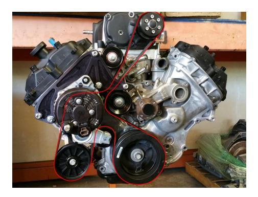
12. Install (3) 8MM flange nuts to secure the alternator bracket to engine.
