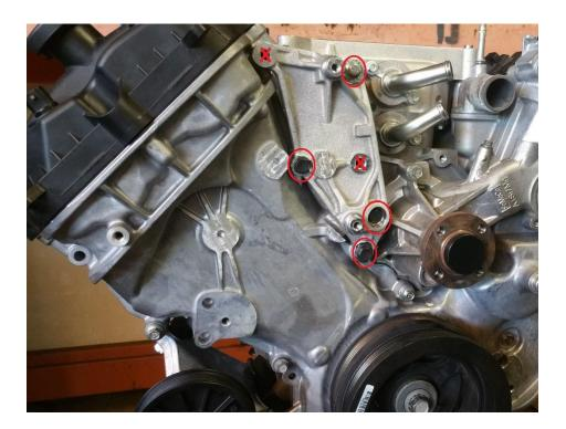
7. Install the three  $\frac{3}{4}$ " hex stand-offs (supplied). The orientation is illustrated in the picture below.
