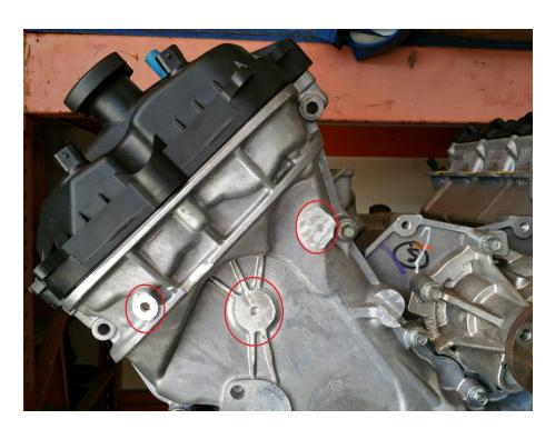
2. Remove half of the stand-off illustrated below. This should be cut down to the height of the bolt boss just below the stand-off (about 3/4" deep).
