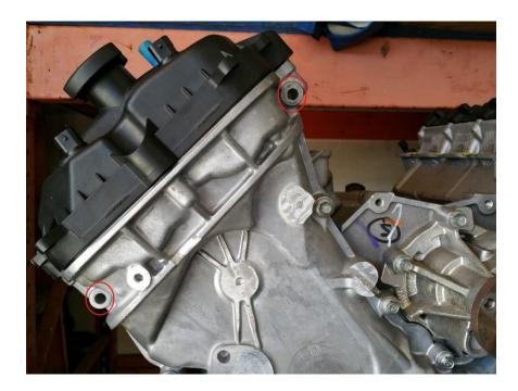
5. Cut the stand-off from the FEAD bracket (supplied with your supercharger kit) as illustrated below. This can be performed with the part on or off engine.
