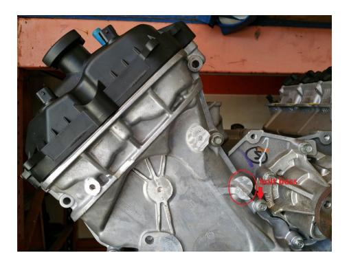
3. Cut a relief into horizontal rib of the timing cover as illustrated below. The center of the cut should be 1/4" deep.
