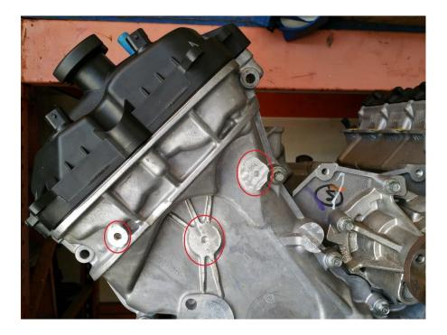
2. Cut a relief into horizontal rib of the timing cover as illustrated below. The center of the cut should be 1/4" deep.
