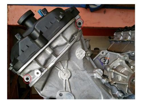
4. Install the three ¾" hex stand-offs (supplied). The orientation is illustrated in the picture below.
