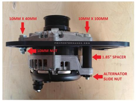
Route the alternator belt (supplied) while installing the assembled alternator bracket leaving the belt off of the A/C compressor pulley. Check clearance between alternator and timing cover. Clearance as necessary.
