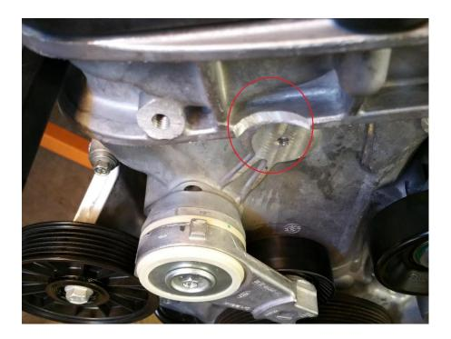
3. Remove the two timing cover bolts as illustrated below.
