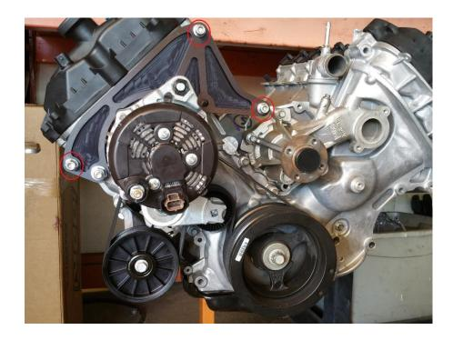
8. Install (3) 8MM flange nuts to secure the alternator bracket to engine.
