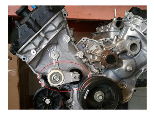
6. Assemble the alternator bracket by attaching the alternator, 1.85' spacer, and hardware as illustrated below. When inserting the 1.85" spacer it may be necessary to press the alternator slide nut out slightly to gain clearance.
