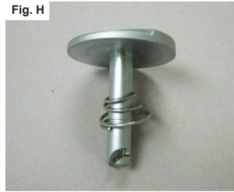
**STEP 8:** Install the factory striker bar with blue locktite. Adjust primary latch until the striker bar fits into the latch. Make sure when the hood is closed you can hear the striker bar "click" into the latch.
