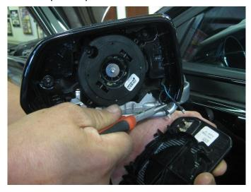
3. Remove the (2) T-15 screws that secure the outer ring to the mirror housing. Use small Screwdriver to release clips, and remove outer ring.
