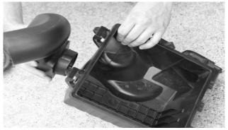
Caution: It is very important that the hole in the air box is precisely cut to 3". We recommend using a 2 3/4" hole saw, then file by hand to achieve proper diameter.
