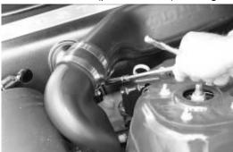
I) Verify Drain Tubes (part #115058) are routed and away from moving parts and hot surfaces.
