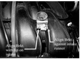
Note: For optimal fitment of "U" clamp, depending on the build date of your vehicle, some cars require trimming of the lip from the bottom side of the intake manifold with a razor blade, this will allow the clamp to fit flat against the manifold.
