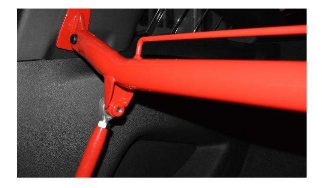
6. Mount harness bar to the upper support plates and connect to the support bars. Adjust the support bars to the desired height.
