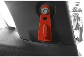
3. Remove the original bolt from the lower seat belt mounting point on both sides. Take off the spacer and washer from the original bolt and set aside the spacer for future use.
