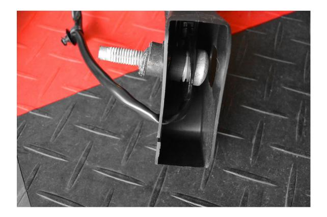
4. Take the original bolt and spacer and assemble them with the harness bar lower support plate as shown.
