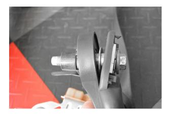
2. Take the original bolt and spacer and assemble them with the harness bar upper support plates as shown.
