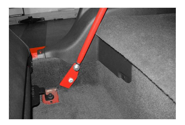
5. Use the smaller additional hole on the lower support plate to mount the provided support bars.
