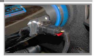
Remove the MAF sensor from the stock air box and install it into the BBK Cold Air Tube using the supplied hardware. (The sensor will only go on one way)
