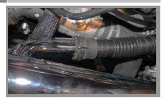
Install the 2 blue couplers to the BBK inlet tube. Install the tube thru the hole in the air filter shield then onto the throttle body. Connect the sound tube to the BBK inlet tube as well.
