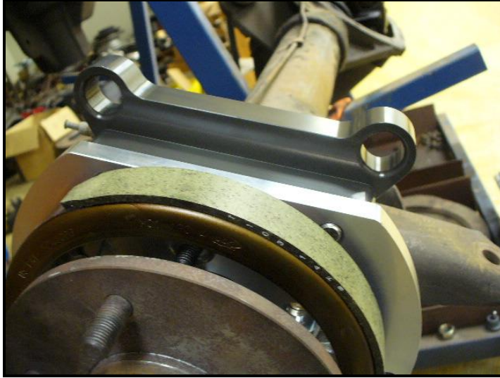
Park brake assembly correctly installed
