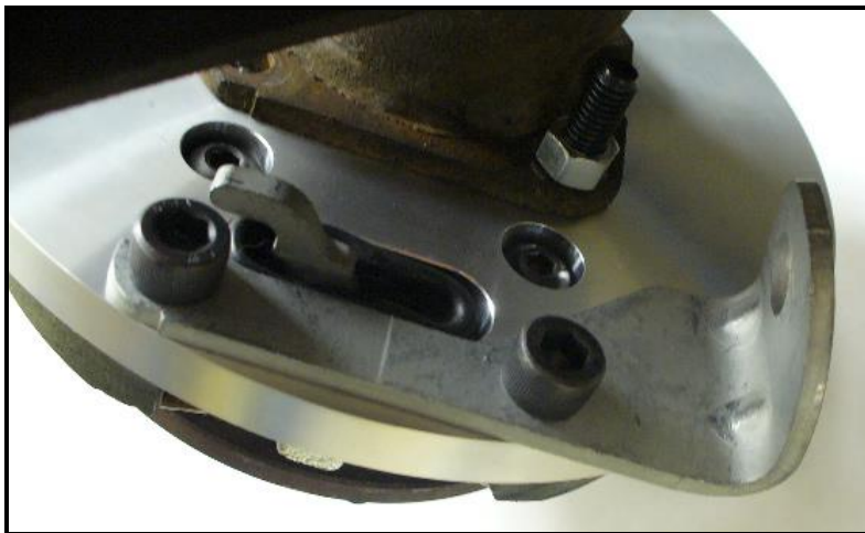
Park assembly installed on driver's side
