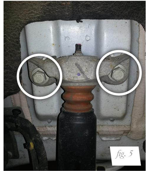
3. Unthread the two upper shock mount bolts and remove the shock from the vehicle.
