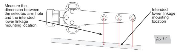
2. Reinstall air lines and cycle the suspension to get to the upper limit position again, measuring between the sensor arm's middle position and directly below the sensor arm hole mounting to the lower linkage ball joint (fig. 18). The difference between these two values will be the full suspension travel range.
