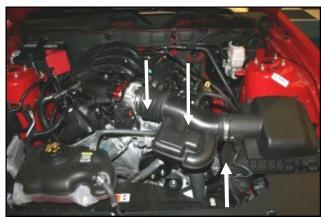
7. Reinstall the intake tube, tighten the two hose clamps, and reconnect the breather line or lines. **Re-connect the negative battery cable!**  Contact your nearest Airaid dealer for an Airaid Intake System for your car, truck or SUV.
