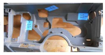
STEP 2: Position gauges as you desire in cluster. Lighly torque down back clamps so you can still adjust from the frontGuages can be placed in any position.
