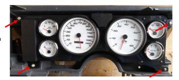
STEP #3 Position brackt and gauges as desired. All holes are slotted/oversize for a great fit for YOUR vehicle. When satisfied, tighter back clamps, re-check and remove from cluster. Wire as neeeded and re-install
