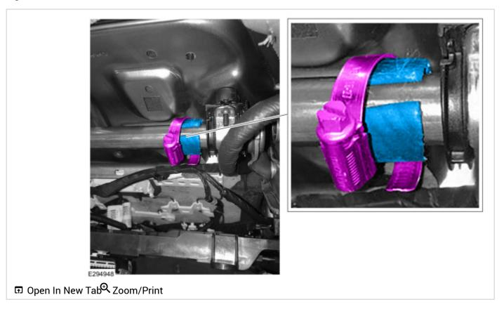
**9.** Push the heater hose up against the handcuff bracket and tighten the hose clamp to 3.7 Nm (33 in-lbs). (Figures 6-9) See Figures 6-7 for clamp orientation.
