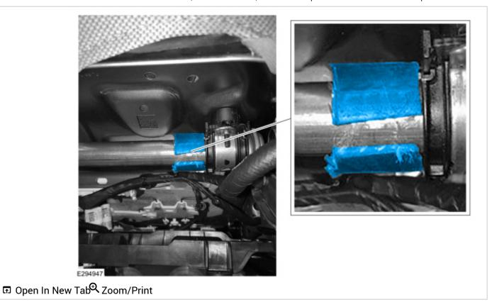
**8.** Open the hose clamp and slip the hose clamp over the heater hose to secure the heater hose to the front cross tube. (Figure 5)
