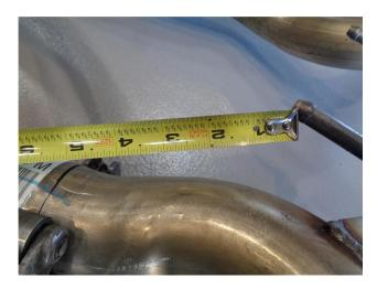
**Step 1.** Begin removing the OEM exhaust system by cutting both pipes exiting the resonator. Measure and cut on the driver side 5" from the tip of the hanger. Cut the passenger side also from the tip of the hanger 5.5" back. Next, extract the hangers from the rubber insulators and remove the OEM mufflers. Retain insulators as they will be used to install the new system.
