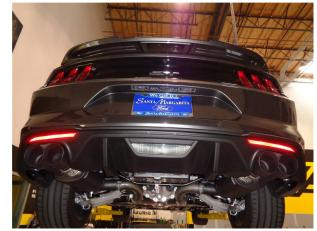
**Step 4.** Once a final position has been chosen for the new exhaust system, evenly tighten all clamps from front to rear using the torque specifications on page one of the instructions. Inspect all fasteners after 25-50 miles of operation and re-tighten if necessary.
