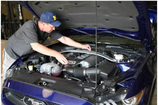
2: Disconnect Mass airflow sensor connector
