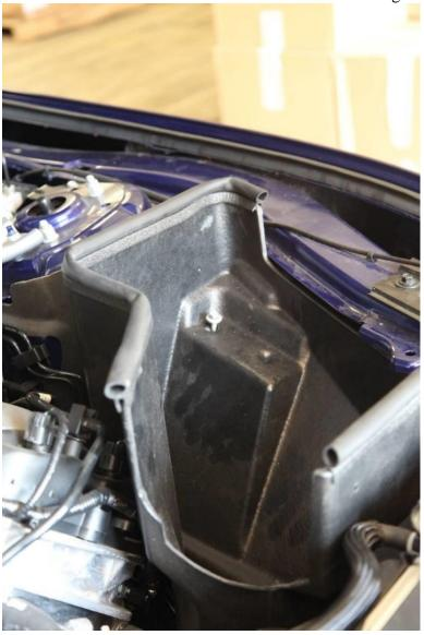
16: Slide large 5" hose coupling onto PMAS intake tube.
