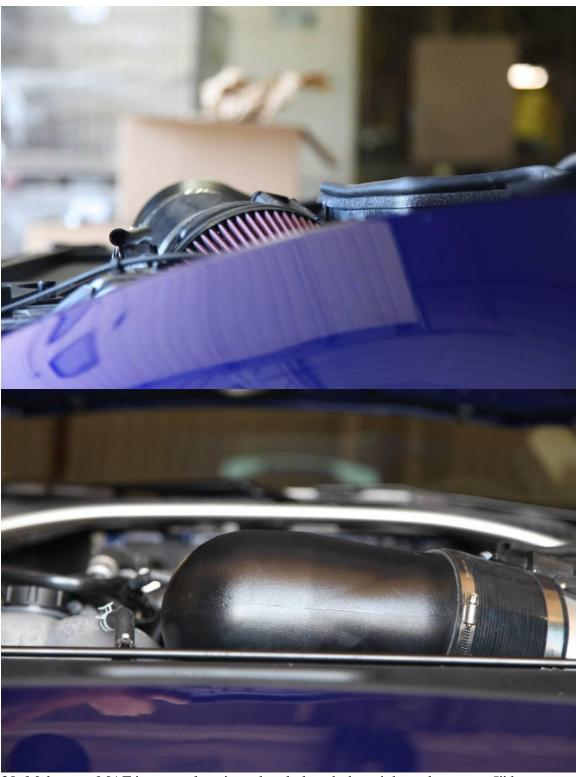
20: Make sure MAF is correctly oriented and placed, then tighten down two 5" hose clamps.
