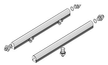
32. Inspect the o-rings on the OEM quick disconnect fitting and replace if necessary. Coat o-rings and the adapter fitting with a light oil and install the AN-06 / Ford quick disconnect adapter fitting on the OEM By-pass fuel line.
