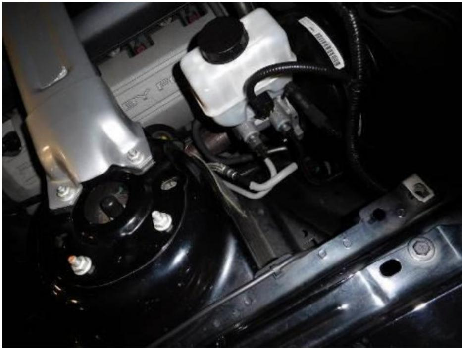
12a: Install supplied sound tube plug into hole in firewall.
