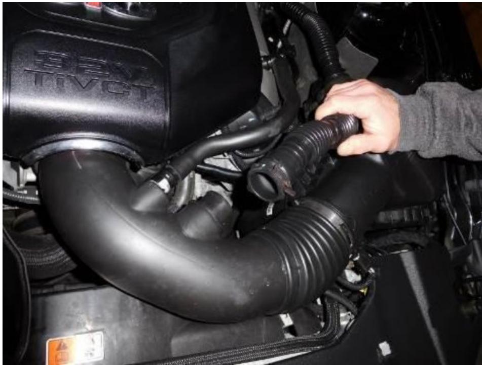
12: Remove intake tube. If desired remove entire sound tube from attachment at firewall.
