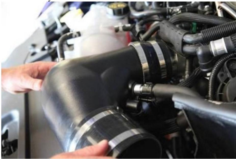
19: This step is very important. Make sure that throttle body coupling is pressed firmly and completely onto throttle body. If done correctly the large intake elbow will be touching the top of the fan shroud, this will ensure proper hood clearance. Tighten throttle body clamp.
